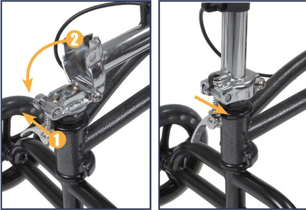
3. Slide locking mechanism into groove on tiller, press locking handle to secure tiller lock in place.
