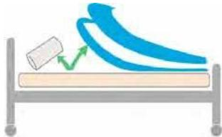
b) On a standard bed, position Mattress Replacement on top of bed, printed top cover facing upwards and air hoses towards the base of the bed. Attach to the bed by securing the adjustable straps under each end of your bed. Ensure buckles are securely fastened and straps are pulled tight. On a profiling bed, secure the side straps around the moveable sections of the bed base.
