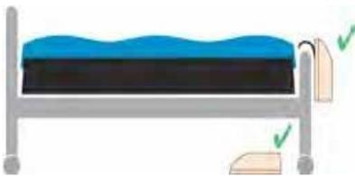
c) On a profiling bed, secure the side straps around the moveable sections of the bed base. **DO NOT SECURE TO THE SIDE RAILS - STRAPS WILL TEAR OFF.**
