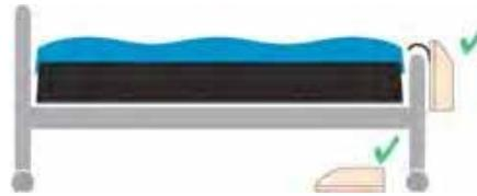
b) Attach the air hoses through the use of the quick connector to the Control Unit. Ensure air hoses do not kink between mattress, bed frame and Pump Unit.
