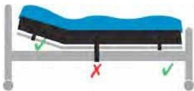
**Important:** Check that the attachment of the Mattress Replacement does not interfere with the movement or operation of the bed.
